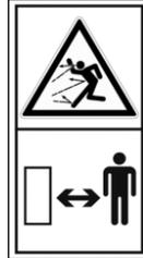
Risk of ejection. Keep unauthorized persons away from the work area while the machine is in use.
